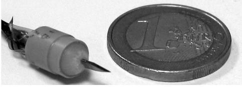
Fig. 2. Picture of the developed force sensing device without the covering cap.
