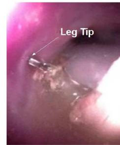
Fig. 16. Capsule opens its legs while immersed in physiological fluids.
