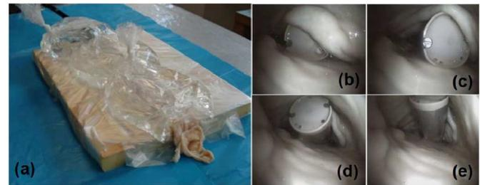
Fig. 15. (a) *Ex vivo* bench test. (b)–(d) Activation of the legged mechanism to get rid of collapsed tissue. (e) Magnetic locomotion starts again after removing the tissue around the capsule.
