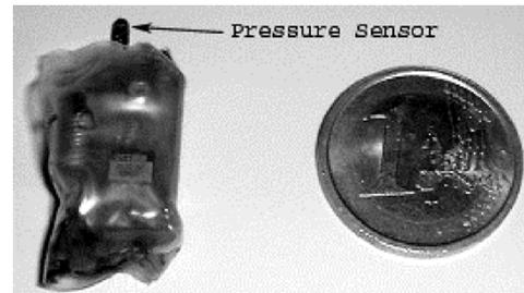
Fig. 6. Transmitter circuit covered with polyurethane film, before silicone embedding.
