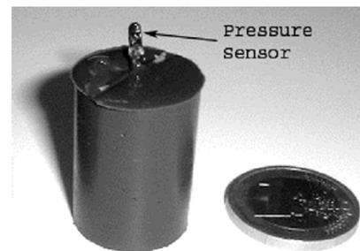
Fig. 7. Photograph of the packaged telemetry system.
