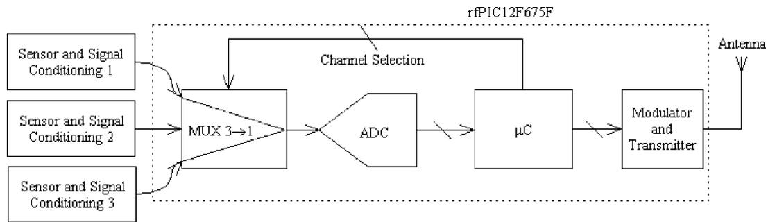
Fig. 4. Implanted circuit block diagram.
