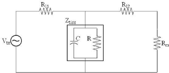
Fig. 3. Equivalent electrical circuit of the whole system.
