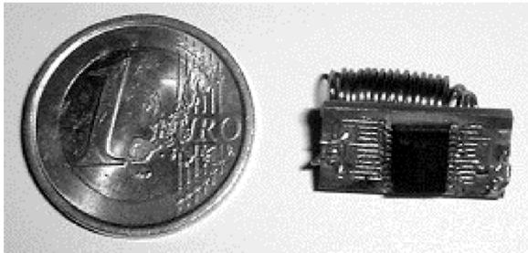
Fig. 5. Photograph of transmitter unit.
