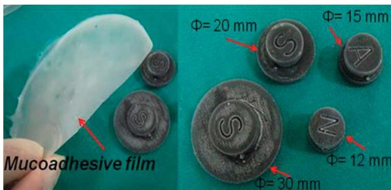
Figure 3. Cylindrical prototyping modules with 12, 15, 20 and 30 mm diameter.
