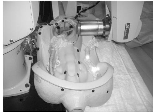
Fig. 15. Experimental procedure with collapsed porcine colon.
