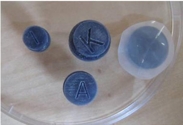
**Fig. 1** Different sizes of prototype passive modules. On the right, the mucoadhesive film (final thickness of 0.2 mm) is attached onto the module base
