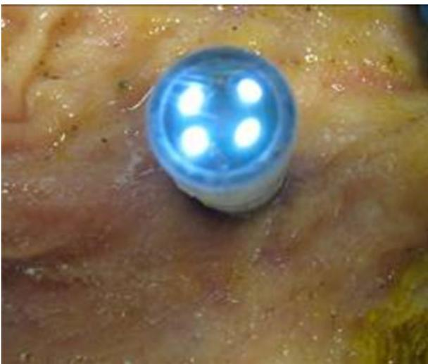
**Fig. 7** Wireless illumination module anchored on the gastric mucosa
