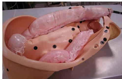
Fig. 2. The experimental setup for exploring how much gas volume is needed to inflate the intestine. Ex vivo porcine intestine was arranged in a phantom model to simulate the shape of the human colon. An endoscope was then used to inject known volumes of air, while the surface area visible on the interior wall was measured in the endoscope images (see Figure 3).
