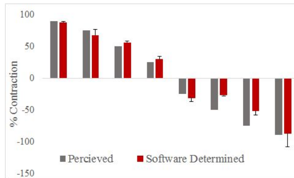
Figure 6: Contraction intent determined by the Software and perceived by the user across multiple test trials
