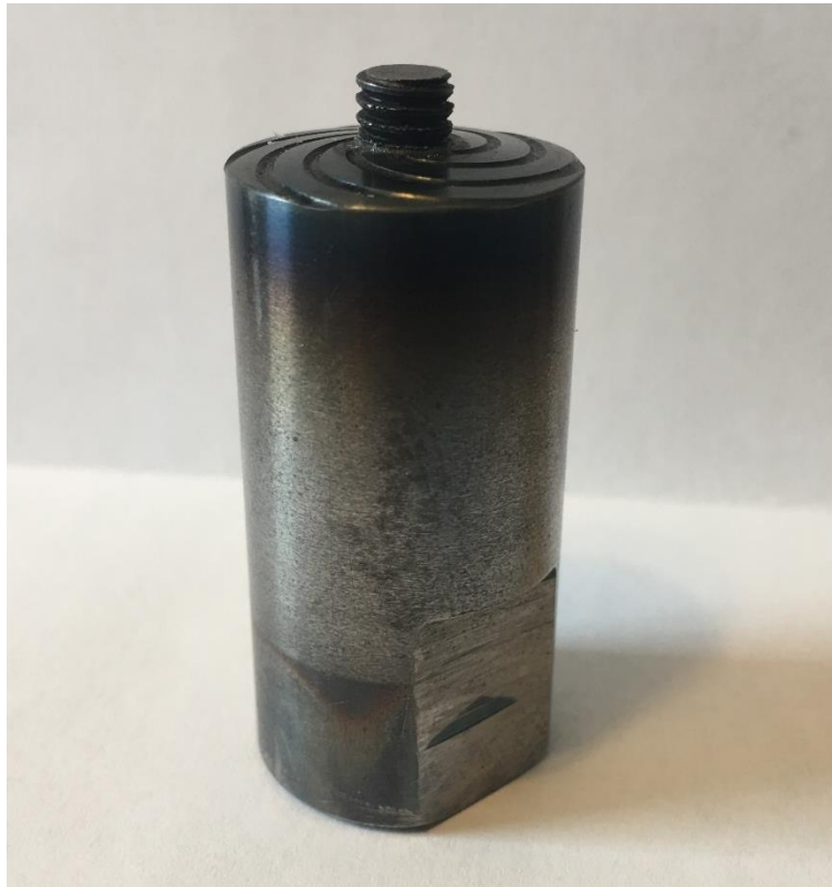
Figure 4 –FSW tool design used for this research featuring a convex scrolled shoulder and threaded pin
