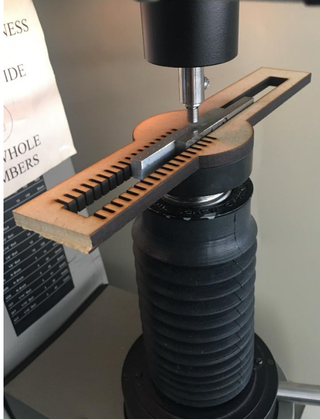
Figure 11 – A sample on the Rockwell hardness tester with MDF testing jig
