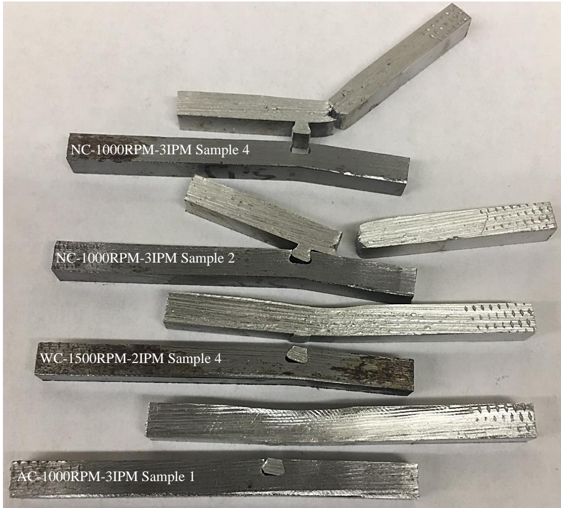
Figure 23 – Tensile shear testing samples. The samples included in this image illustrate the variability of failure during shear testing. From top to bottom the samples pictured are sample 4 from NC-1000RPM-3IPM, sample 2 from NC-1000RPM-3IPM, sample 4 from WC-1500RPM-2IPM, and sample 1 from AC-1000RPM-3IPM.
