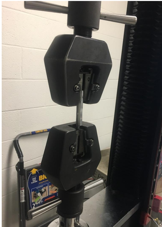
Figure 12 – A sample on the Instron tensile tester
