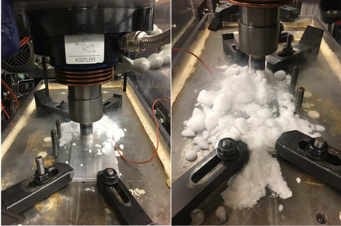
Figure 8 – (Left) The DI weld with the FSW tool traversing towards the camera. (Right) The trailing end of the DI weld which shows DI piled onto the weld using a tablespoon measurer.
