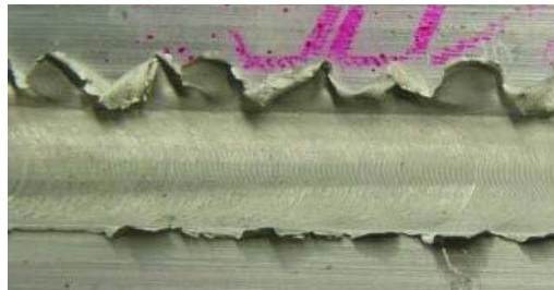
Figure 15: Typical weld deformation for overheat phenomena experienced during experimentation. (Parameter Set: 3750 rpm and 27.7 ipm.)
