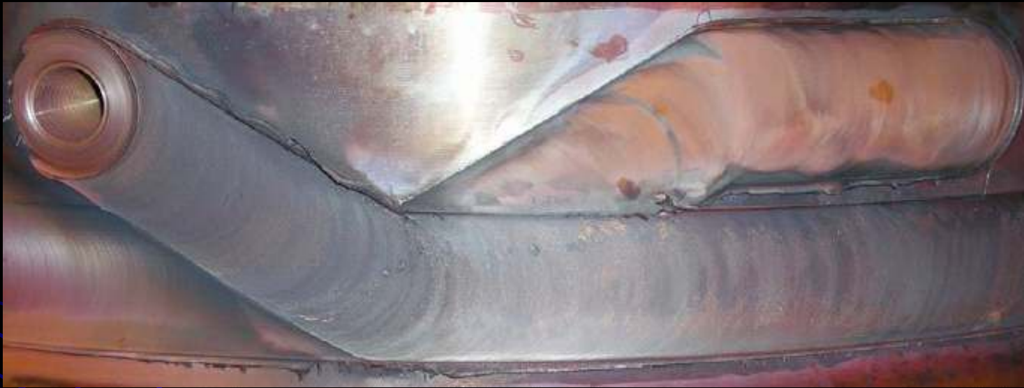
Figure: 'Start and park' method in the welding of cylinders without a RPT [2.]
