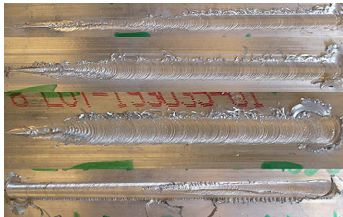
Fig. 15. Attempts a probe tapered retraction from 1/8 in. material full penetration welds at various parameters. The probe tends to ‘drag’ through the material near exit.
