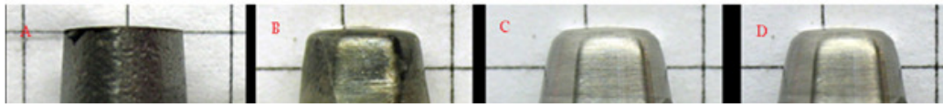
Figure 3. Evolution of wear for 2000 RPM, 7 IPM. A) original probe B) after 8 inches of weldment C) after 16 inches of weldment D) after 24 inches of weldment.
