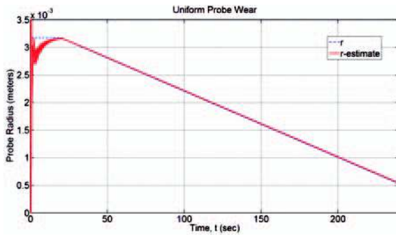
Fig. 11 Estimation of uniform probe wear
