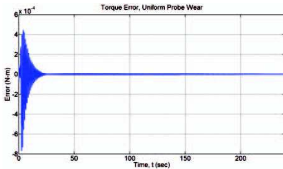
Fig. 12 Torque error while simulating uniform probe wear
