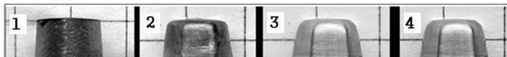
Fig. 2 Progressive tool wear on MMC at 2000 r/min, 7 inches/min: (1) new probe; (2) 8 inches of weld; (3) 16 inches of weld; and (4) 24 inches of weld
