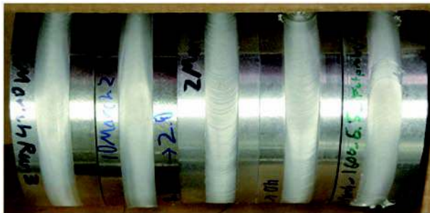
Fig. 11 The superficial appearance of several pipes welded in the experiment
