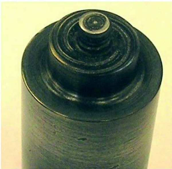
Fig. 9 The 5/8" (15.9 mm) diameter scrolled shoulder, 3/16" (4.8 mm) probe diameter tool used in this experiment. The scrolled shoulder feature increased tolerance to variation in contact condition and improved weld appearance
