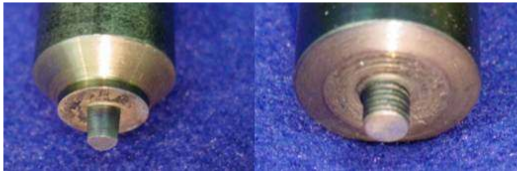
Figure 3.3: Trivex and threaded FSW tool.
