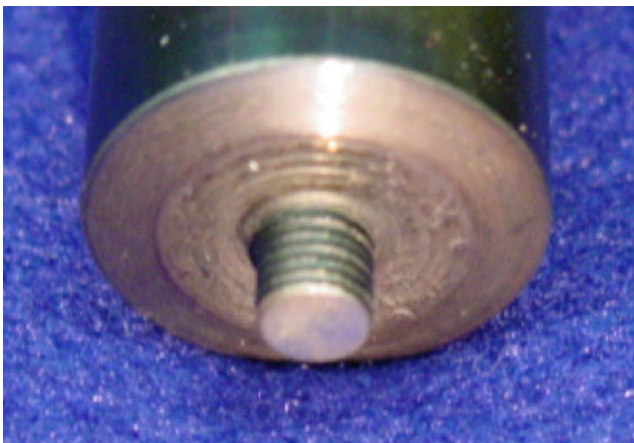
Fig. 4 FSW tool used for torque control
