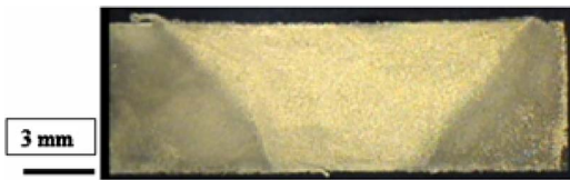
Fig. 18 Weld using 1/4 in. Trivex tool and force control via traverse speed
