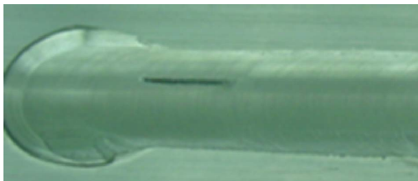
Fig. 8 Weld flaw due to lack of force control
