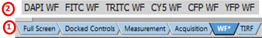
1. Choose WF tab **1** at the bottom of screen, and choose optical configuration **2** at the top of the screen to match your fluorophore of interest.
