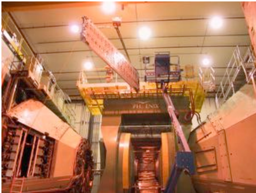
FIGURE A.1. TOFW Sector Installation (PHENIX IR)
