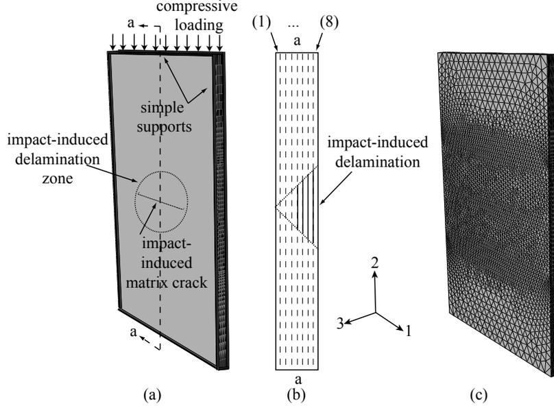
Figure 3: The numerical model of the CAI specimen: (a) boundary conditions and impact-induced damage, (b) impact-induced delamination along the thickness direction, and; (c) finite element discretization of the CAI specimen.
