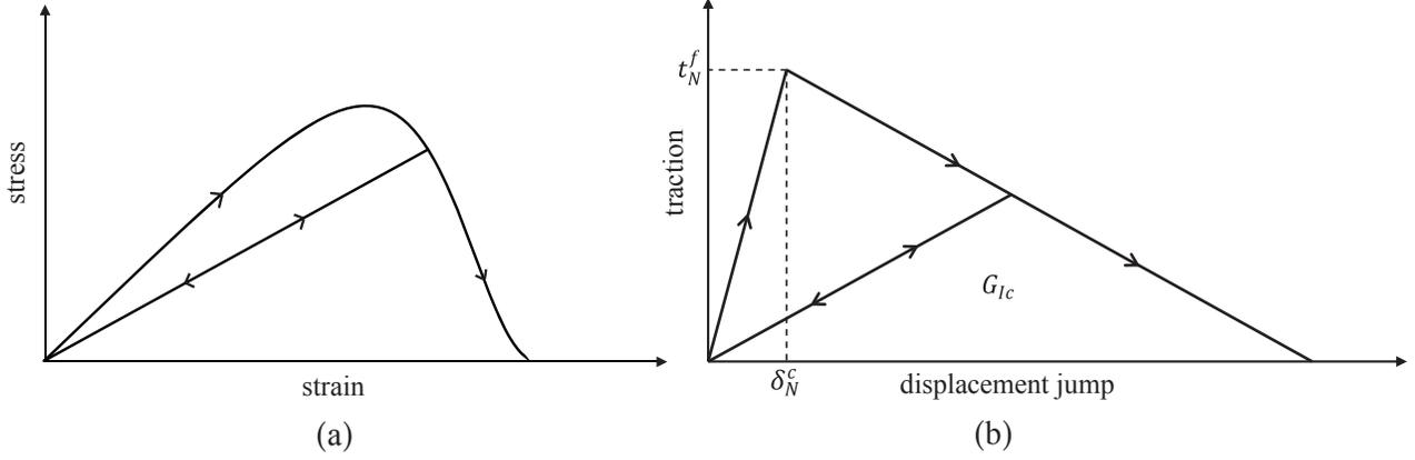
Figure 5: Illustration of the damage progression models: (a) bilinear cohesive law for delamination propagation in case of pure mode I condition. A mixed mode cohesive surface law is employed in the simulations, (b) damage evolution law for composite constituents.
