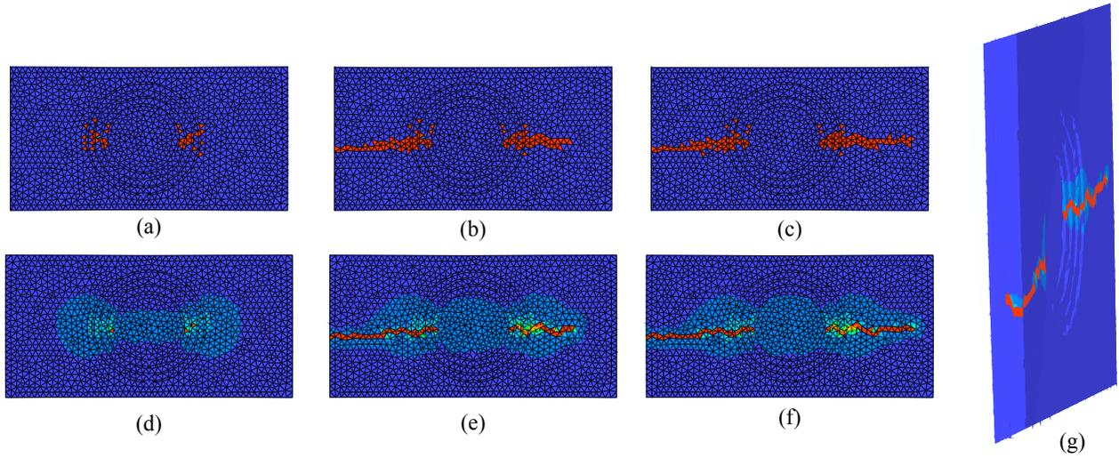
Figure 9: Damage propagation in the composite constituents upon sublaminar buckling (a)-(c) propagation of matrix damage; (d)-(f) propagation of warp fiber damage; (g) shear crack propagation causing ultimate failure. The middle third of the specimen is shown (back face).
