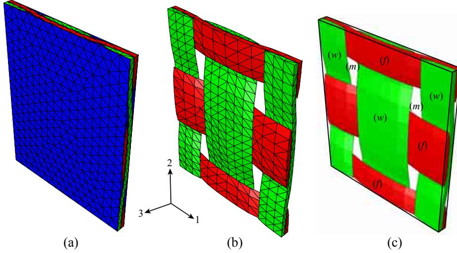
Figure 4: The representative volume for the woven composite material (a) finite element discretization; (b) finite element discretization of the fibers, and; (c) Reduced order model for the RVE with three constituents: fill (horizontal) and warp (vertical) fibers and the matrix (transparent).
