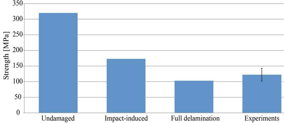
Figure 7: Experimental and simulated sublaminates buckling strength of composite specimens.
