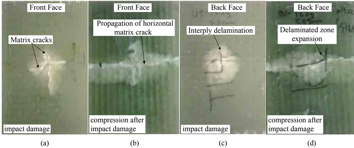
Figure 1: Damage profiles: (a) Impact-induced damage profile viewed from the front (impacted) face, (b) damage profile after compression loading viewed from the front face, (c) Impact-induced damage profile viewed from the back face and (d) damage profile after compression loading viewed from the back face.
