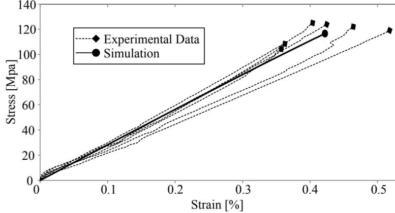
Figure 10: CAI Stress-strain diagram of the composite specimen based on numerical simulations and experiments.
