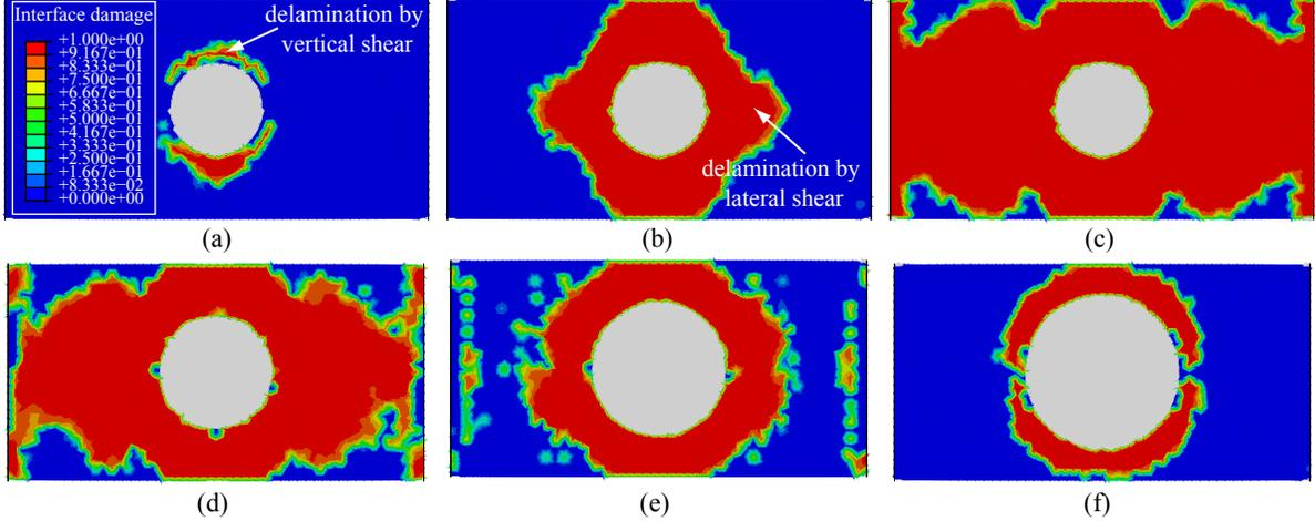
Figure 8: Interface damage profiles between: (a) 4th and 5th plies under 29 MPa compression; (b) 4th and 5th plies under 86 MPa compression; (c) 4th and 5th plies under 138 MPa compression; (d) 5th and 6th plies under 138 MPa compression; (e) 6th and 7th plies under 138 MPa compression, and; (f) 7th and 8th plies under 138 MPa compression.
