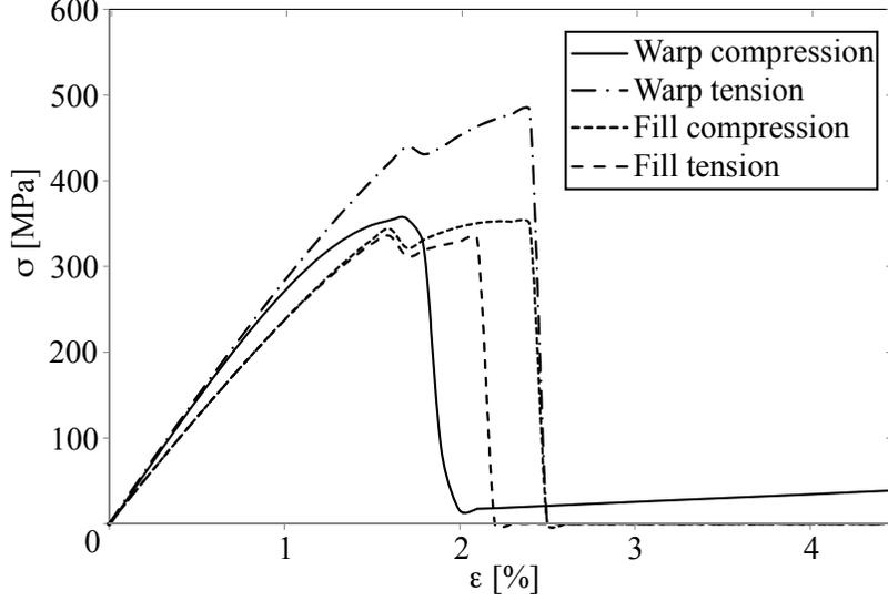
Figure 6: The stress strain response of the composite RVE along the fill and warp directions under compressive and tensile loading.
