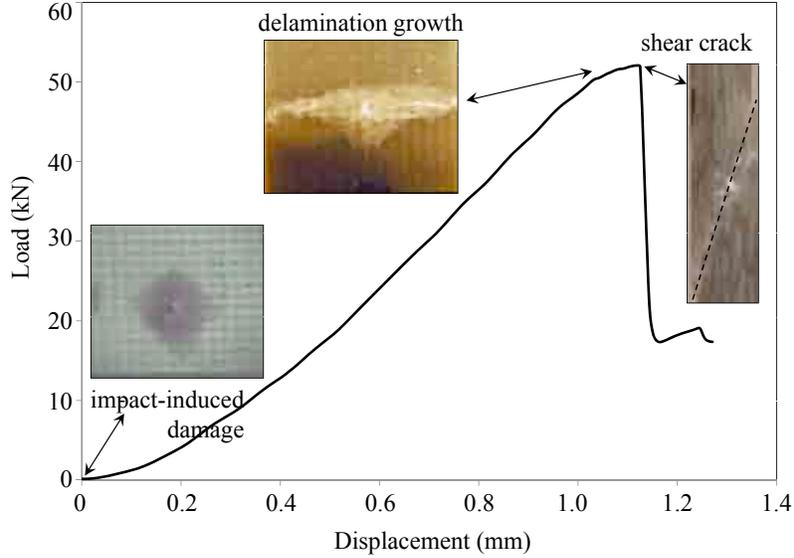
Figure 2: A schematic of the load-displacement curve of an impacted composite laminate in compression.
