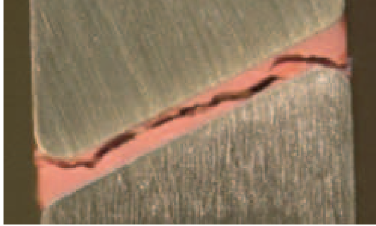
Figure 10: Crack path of the RME adhesive layer after a monotonic uniaxial tensile test. Courtesy of the National Physical Laboratory, UK.
