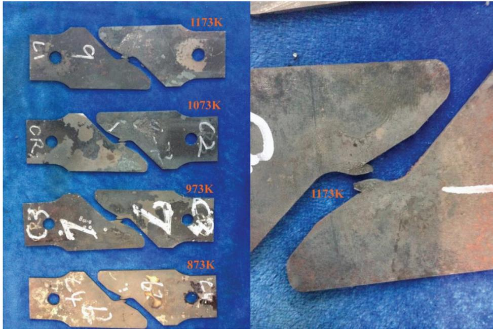
Fig. 21 Final fracture morphology in shear specimens of 22MnB5 steel at different temperatures
