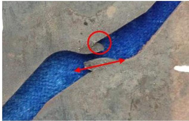
Fig. 25 The experiment of the local middle part of the 22MnB5 specimen at 1173 K (arrow representing for the fracture direction and the circle showing the position of severe deformation)
