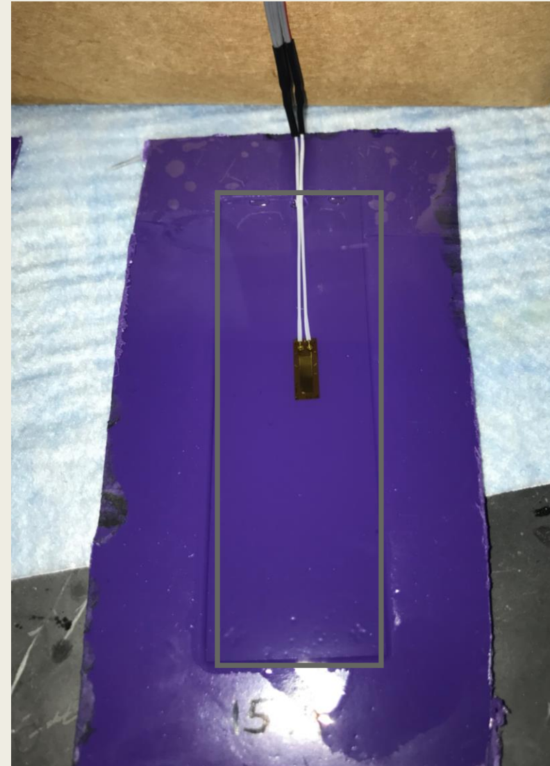
Wired strain gauge curing in 15:1 PDMS
