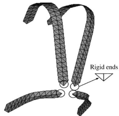
Fig. 5 FEM belt model
