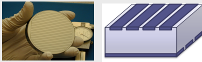
Left: Image of HPGe DSSD crystal. Right: Schematic of DSSD configuration [4], our detector is similar, only round.
