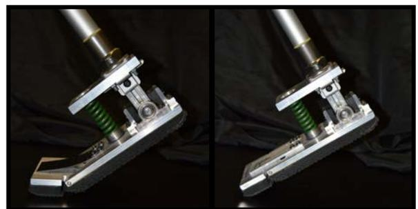
**Figure 1:** Prosthetic foot with adjustable ankle and toe joint stiffness. We compared walking with an elastic toe joint (left) vs. without (right; rigid strut inserted across joint to prevent toe rotation).
