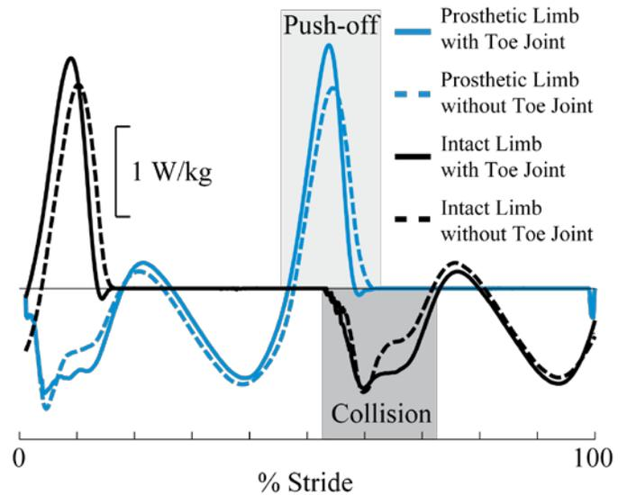
**Figure 2:** COM power for the prosthetic and intact limbs, for a representative subject. Inclusion of a toe joint led to increased peak Push-off power during walking.
