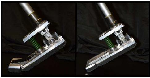
Figure 1: Prosthetic foot with adjustable ankle and toe joint stiffness. We compared walking with an elastic toe joint (left) vs. without (right; rigid strut inserted across joint to prevent toe rotation).
