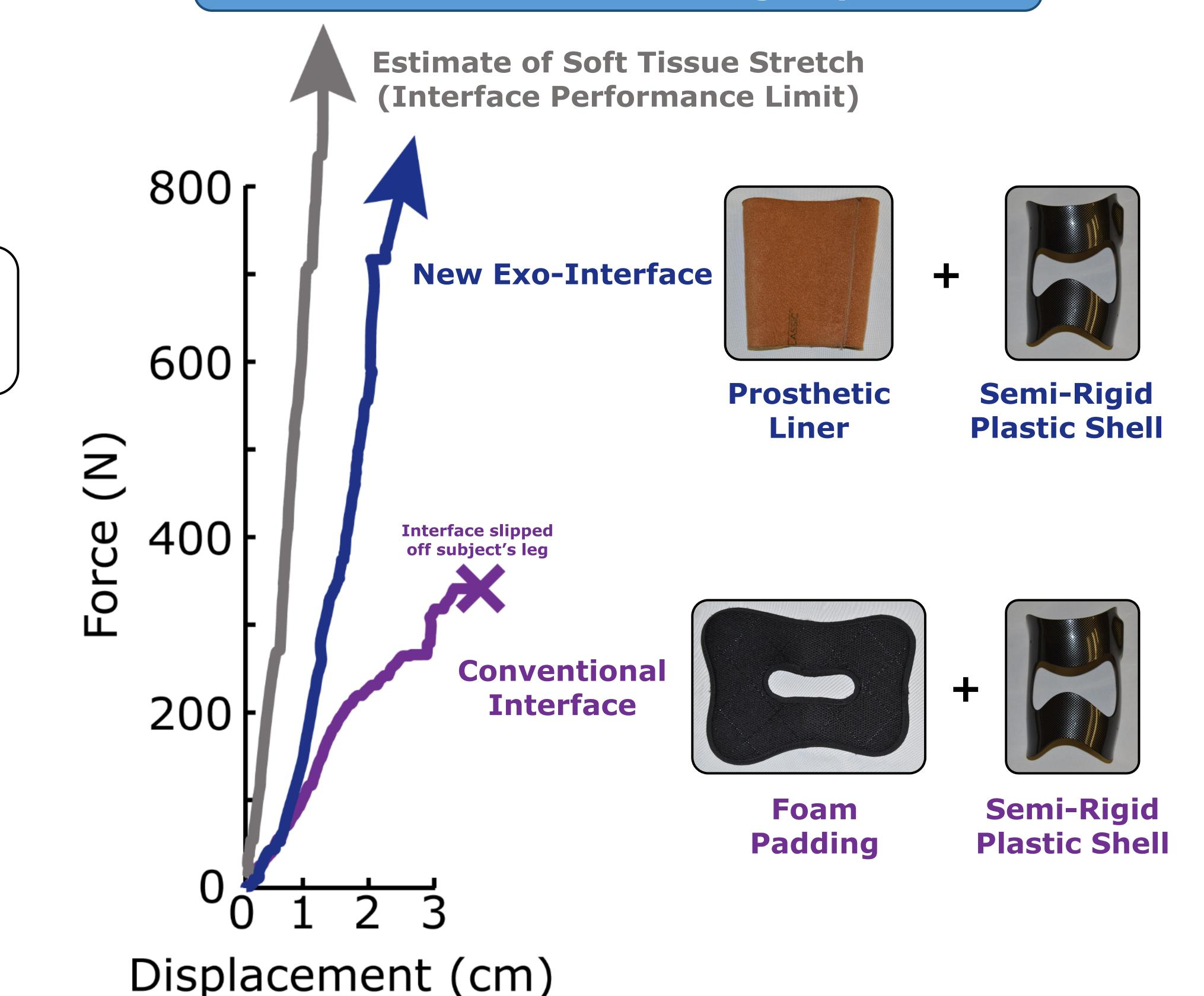
Novel Interfaces could Overcome Current Limitations, Enhancing Exoskeleton Benefits by Improving Force and Power Transfer to the User
