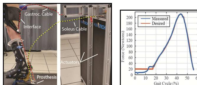
Figure 1: Experimental Set-up (left), Stiffness Emulation (right).
