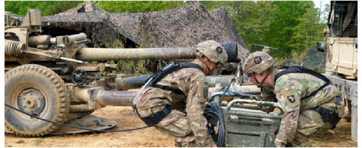
Soldiers wear the Soldier Assistive Bionic Exosuit for Resupply to assist with lifting. (Vanderbilt University)
