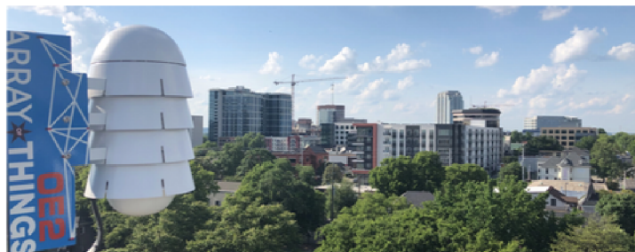
Array of Things sensors can measure air quality and other environmental factors. (Vanderbilt University)
