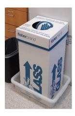
This is a well-maintained box with the bag/liner properly installed and a tray to protect the bottom.
