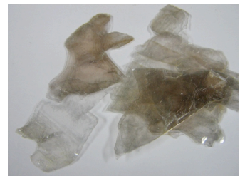
Above: The mineral muscovite cleaves into thin sheets.
