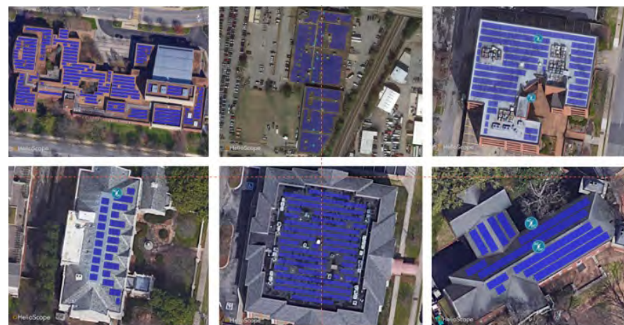
Figure 13. Example of On-site Solar Analysis Layouts on Selected Buildings
