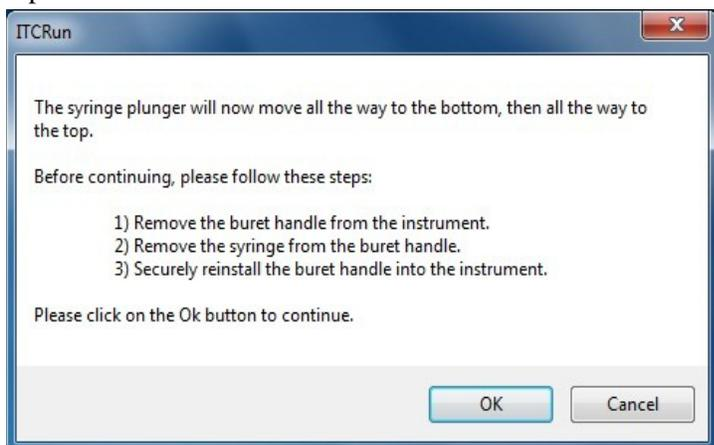
After the buret drive stops moving, it will be located at the top position and the buret position will be reported as 100% on the top of the NanoITC screen.
