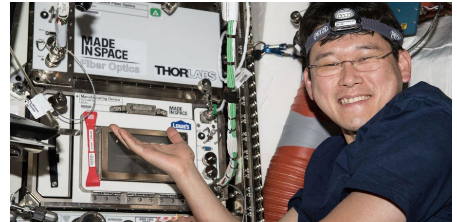
Made In Space Fiber Optic draw apparatus on the International Space Station
