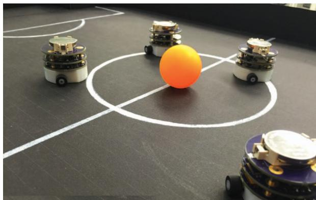
**Figure 5.** Four eSMAC robots playing two-on-two robot soccer with a table-tennis ball.
