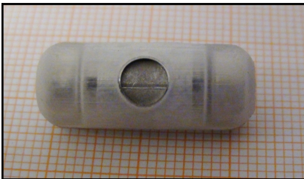
Fig. 15 Assembled biopsy capsule prototype laying on graph paper for reference
