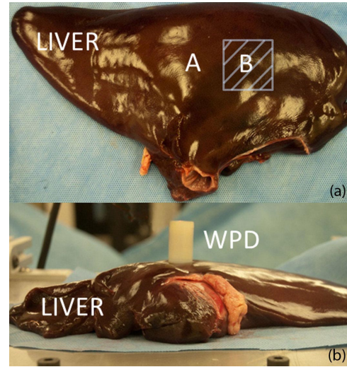
Fig. 8. Liver sample where A and B highlight the positions where wireless palpation was performed. The squared lump was embedded 10 mm beneath the tissue in position B, as represented by the squared overlay. Distance between position A and B is 20 mm (a). Side view of the porcine liver with the WPD above position A (b).
