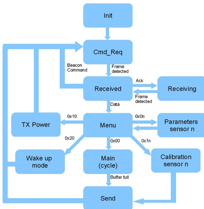
Fig. 4. Flow diagram of the implantable unit firmware.
