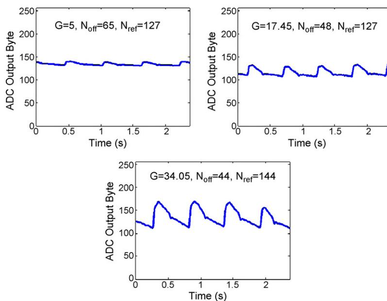
Fig. 5. Calibration procedure: sequence of acquisitions increasing the gain in order to match the signal dynamics. The INA321 gain ( $G$ ), the offset rejection ( $N_{\text{off}}$ ) and the zero line ( $N_{\text{ref}}$ ) are indicated for each subplot.
