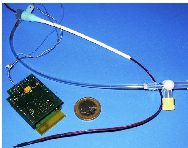
Fig. 3. Implantable unit before packaging.
