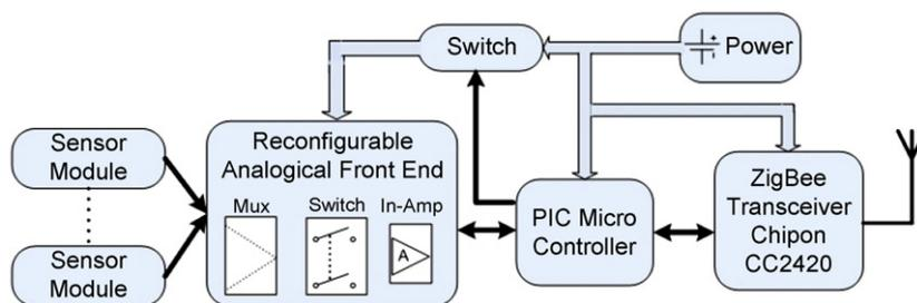
Fig. 1. Block diagram of the implantable unit.
