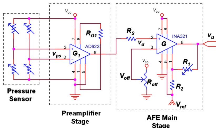
Fig. 2. AFE configuration for pressure measurements.
