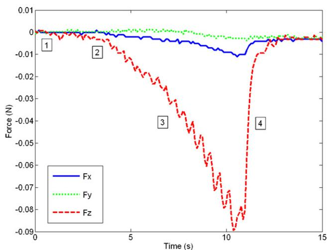
Fig. 12. Force signals from the reference load cell during the different phases of cell palpation.
