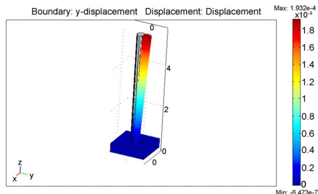
Fig. 4. Boundary plot of the sensor displacement in the y direction in response to a 0.1 N tangential loading at the tip.
