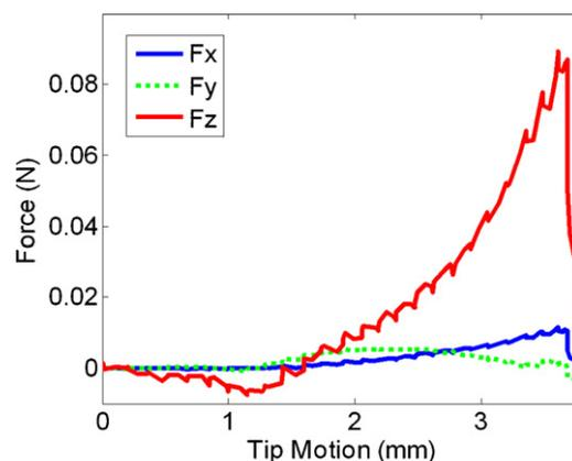
Fig. 13. Force signals from the reference load cell during the different phases of cell palpation.
