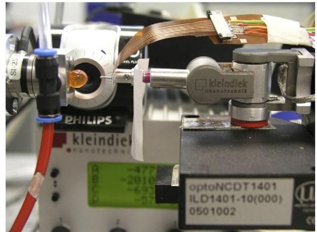
Fig. 9. Cell palpation and injection setup.
