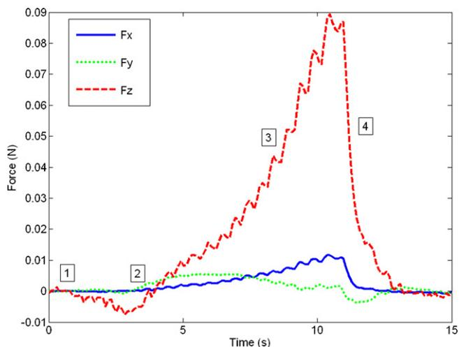
Fig. 11. Force signals from the force sensor during the different phases of cell palpation.
