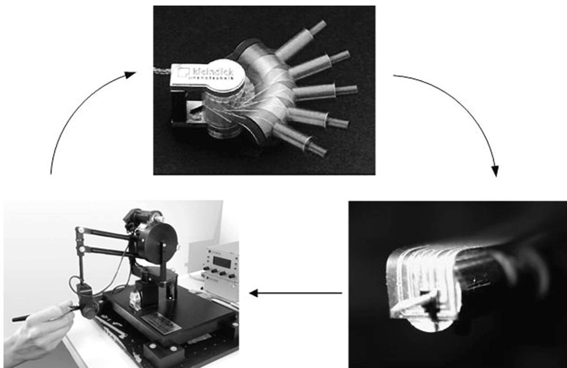
Fig. 7. Bilateral manipulation platform with triaxial force feedback.
