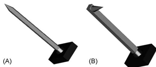
Fig. 2. Axial tip (A) and flat tip with a dedicated probing end bonded onto the sensor (B).
