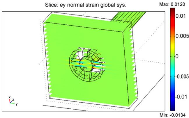
Fig. 5. Slice plot of the y component of normal strain in response to a 0.2N tangential loading at the tip.
