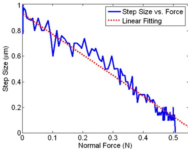
Fig. 8. Nanomanipulator step size versus the force on the tip.
