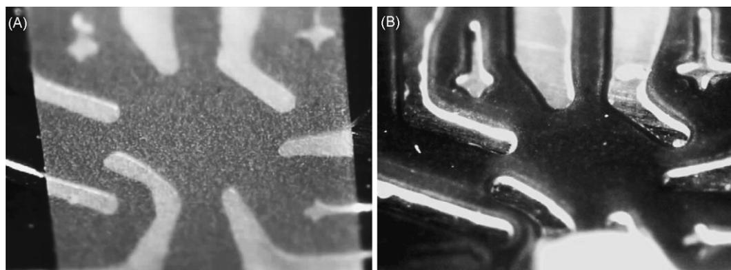
Fig. 7. (A and B) Tacking the film to the substrate.
