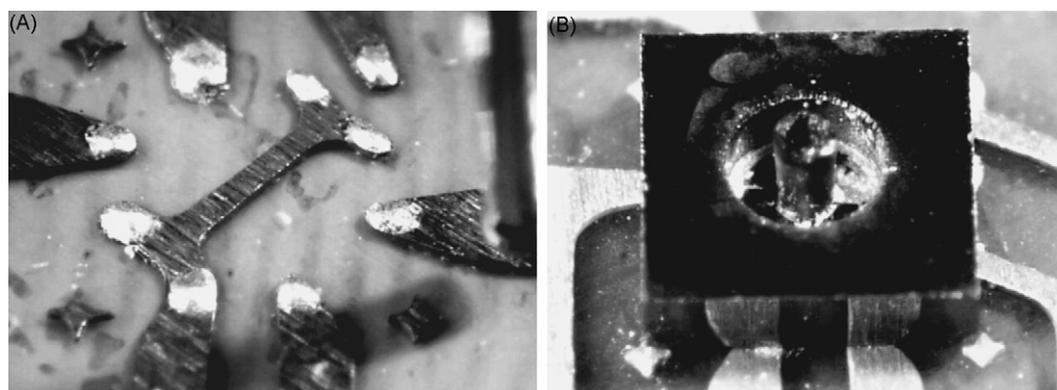
Fig. 5. (A) Dispensing, (B) placed sensor.
