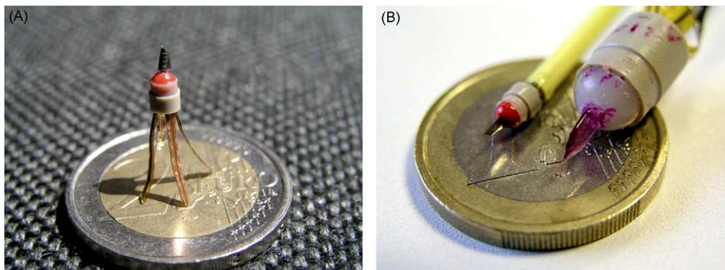
Fig. 13. (A) Sensorized cutting device for surgical applications with the triaxial force sensor as core component. The flexible circuit tracks that come out of the sensor housing lead directly to the MEMS sensor which is placed under the nylon ball encapsulated in soft polyurethane. (B) Direct comparison of the miniaturized tool (left) with the previous one (right) demonstrates the advantage of a direct assembly of the force sensor on a flexible circuit.
