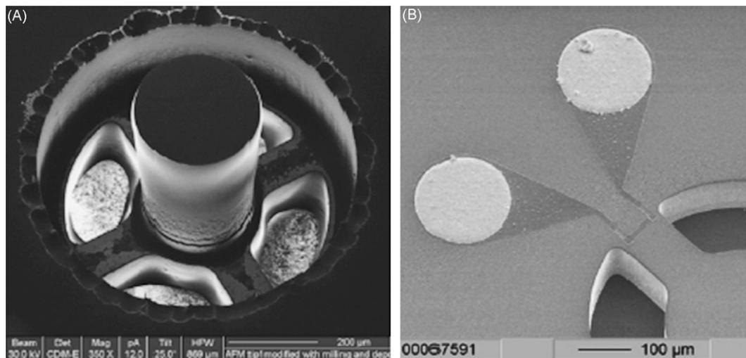
Fig. 1. (A) FIB image of the sensor, (B) piezoresistors and pads.
