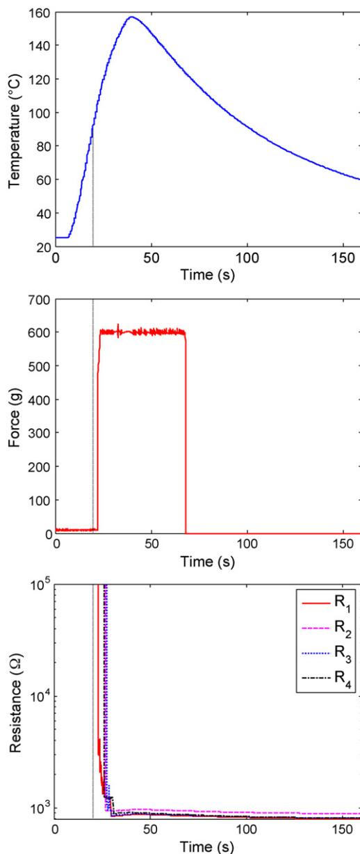
Fig. 9. (A–C) Temperature, force and resistances during the assembly process.
