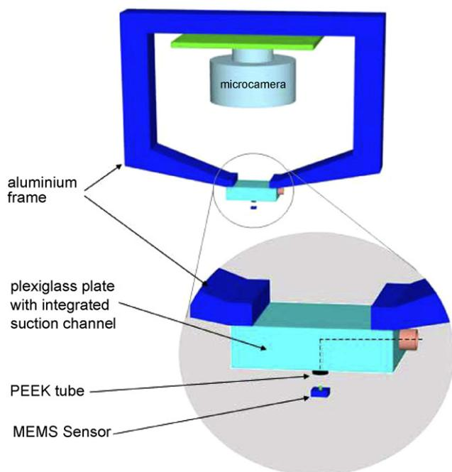
Fig. 14. Design of the new vacuum gripper with an integrated microcamera.
