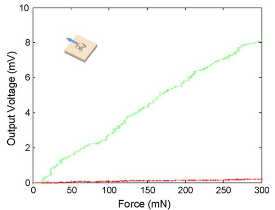
Fig. 12. Output voltage for tangential loadings.
