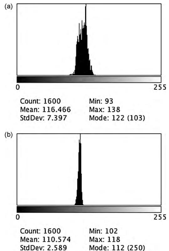
Fig. 9. Histogram of PILLCAM SB2 image selected region (a) and of the proposed camera module selected region (b).
