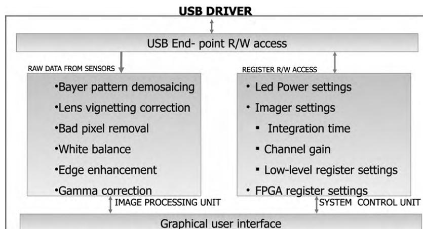
Fig. 4. Software architecture of the demonstration system.
