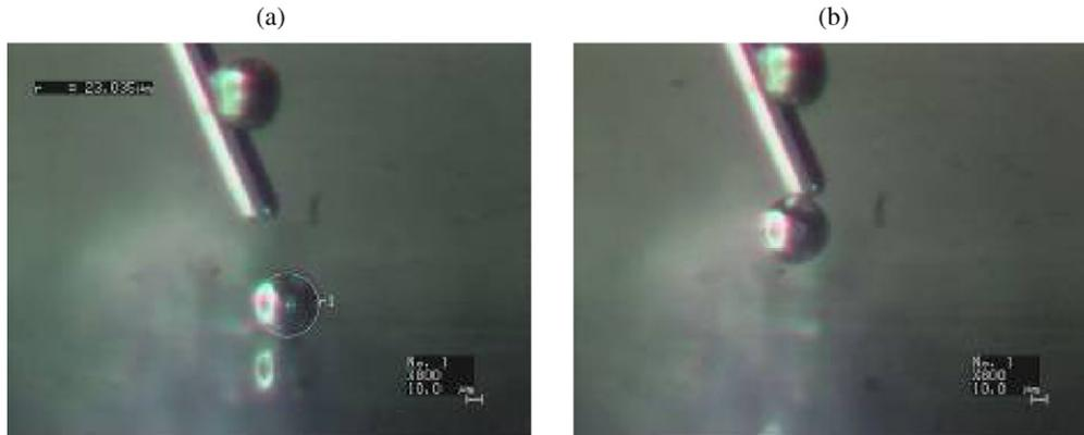
Fig. 6. A 23 μm spherical object before (a) and after (b) grasping by using 20 V with a relative humidity of 10%.
