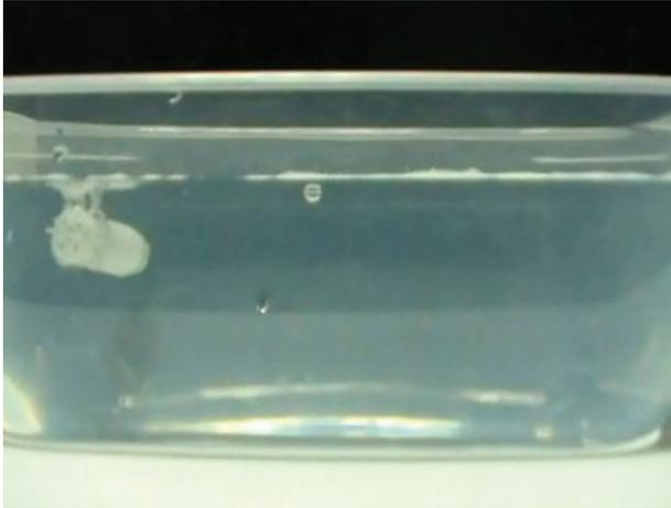
Figure 7. Neutral buoyancy with idle motors.
