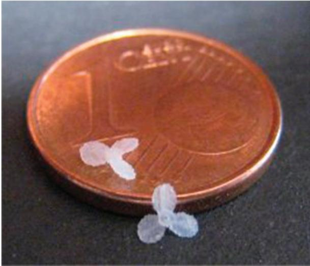
Figure 4. Prototypes of three-blade propellers.
