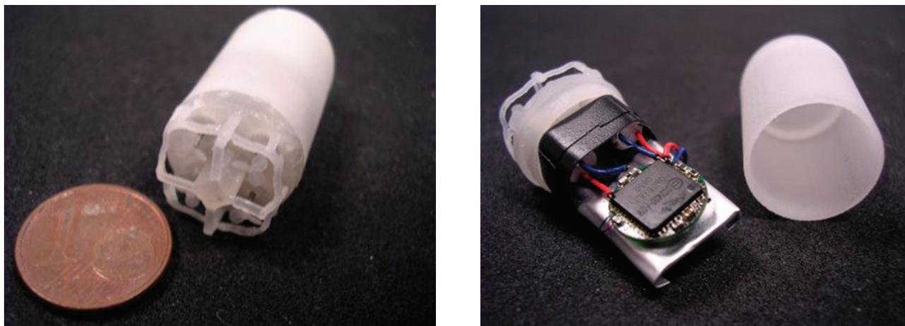
Figure 5. Assembled capsule (left); view of the internal components (right).
