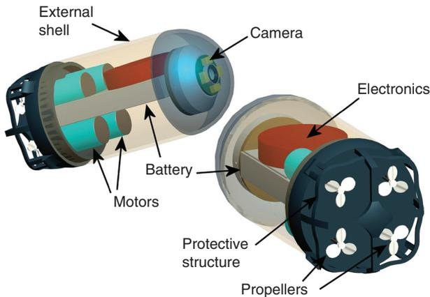
Figure 3. 3D sketch of the capsule and its internal components.
