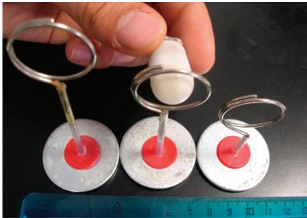
Figure 8. Detail of the ring-shaped targets and comparison with the capsule.
