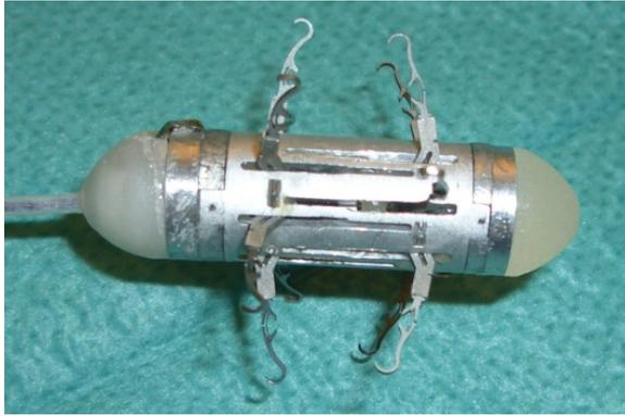
**Figure 1.** The assembled endoscopic capsule robot that is the focus of our case study. Its internal components are shown in figure 3.
