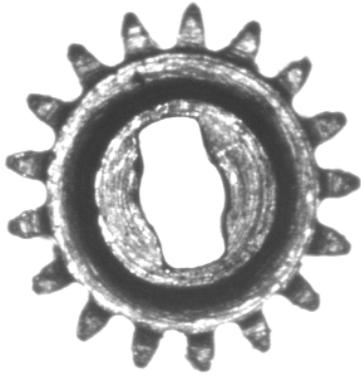
**Figure 16.** The brass gear. The design value for the addendum radius is 1.140 mm.
