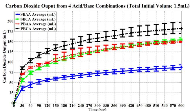
Fig. 6. The carbon dioxide generated by the four combinations of potassium bicarbonate (PB), sodium bicarbonate (SB), acetic acid (AA), and citric acid (CA). The average output is presented as a line, and the minimum and maximum values are presented with error bars. From this, we observe that the PB+CA reaction generated the most gaseous output.
