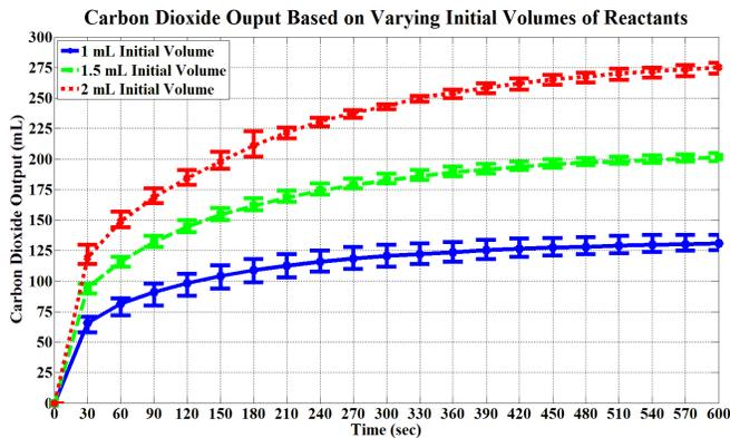
Fig. 8. The carbon dioxide produced by varying total initial volumes of reactants (potassium bicarbonate, citric acid, and water). The average output is presented as a line, and the maximum and minimum values are presented with error bars. From this, we observe that a larger initial volume produces a larger gaseous output, following a linear relationship.
