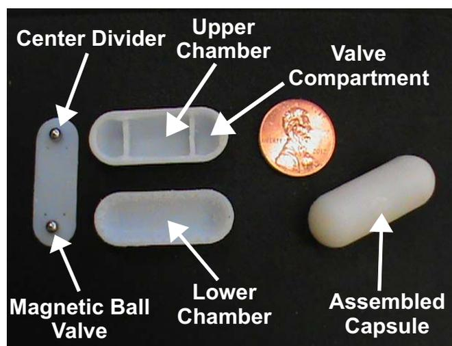
Fig. 10. The capsule prototype and its components. The upper chamber is designed to hold the acid solution, while the lower chamber holds the powdered base. In the presence of an external magnetic field, the two magnetic ball valves move toward the top of the upper chamber, and the citric acid solution mixes with the potassium bicarbonate. The  $\text{CO}_2$  produced is vented through small perforated holes just under the midline of the capsule.
