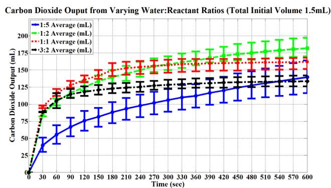
Fig. 7. The carbon dioxide generated by varying ratios of water to reactants for potassium bicarbonate and citric acid. The average output is presented as a line, and the maximum and minimum values are presented with error bars. From this, we observe that the 1:2 water:reactant ratio produced the most gaseous output.
