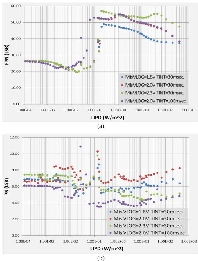
Fig. 7. (a) FPN and (b) PN at different  $V_{LOG}$  and  $T_{INT}$  values over the whole LIPD range.
