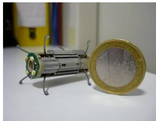
Fig. 1: Capsule without plastic cover. The capsule is equipped with legged locomotion and illumination. Capsule size is 10mm x 33mm.
